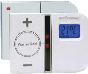
AS2-RF thermostat transmits via Z wave mesh radio technology and is capable of operation in most domestic houses with an operating range of approximately 30 metres. Ideal for controlling combi boilers, it can be mounted in any suitable location without the need to disturb existing wiring or décor. Operates from 3 standard AA batteries, with 2 years+ life and separate clock battery.
