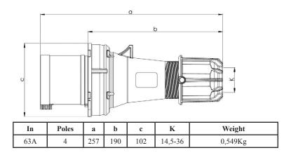
Our IEC/CEE connectors are now tested and certified under the international standard IEC 60 309, which has been developed in the IEC standardisation organisation (International Electrotechnical Commission). This worldwide standard is systematically applied to all GARO products. The use of this standard eliminates the possibility of incorrect connections, regardless of the circumstances.
