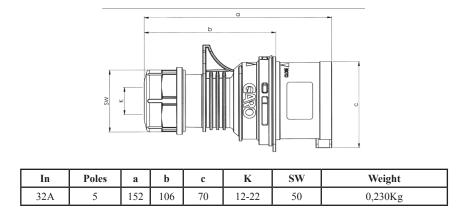
Our IEC/CEE connectors are now tested and certified under the international standard IEC 60 309, which has been developed in the IEC standardisation organisation (International Electrotechnical Commission). This worldwide standard is systematically applied to all GARO products. The use of this standard eliminates the possibility of incorrect connections, regardless of the circumstances.
