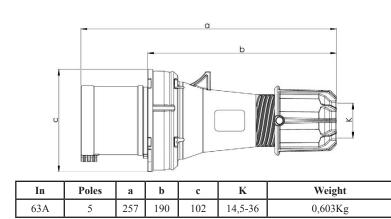
Our IEC/CEE connectors are now tested and certified under the international standard IEC 60 309, which has been developed in the IEC standardisation organisation (International Electrotechnical Commission). This worldwide standard is systematically applied to all GARO products. The use of this standard eliminates the possibility of incorrect connections, regardless of the circumstances.
